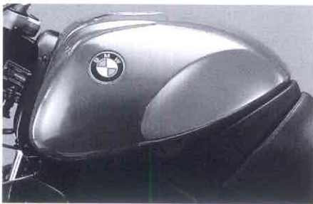
Elegantly shaped: the new BMW sheet-steel tank holds a generous 21 litres of fuel.
